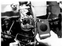
Fig. 8-20 (A) Timing tester (09900-27003)
