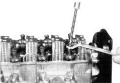
Fig. 3-152 Adjusting valve clearance
