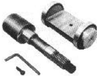
09924-36320 Bevel pinion mounting dummy
