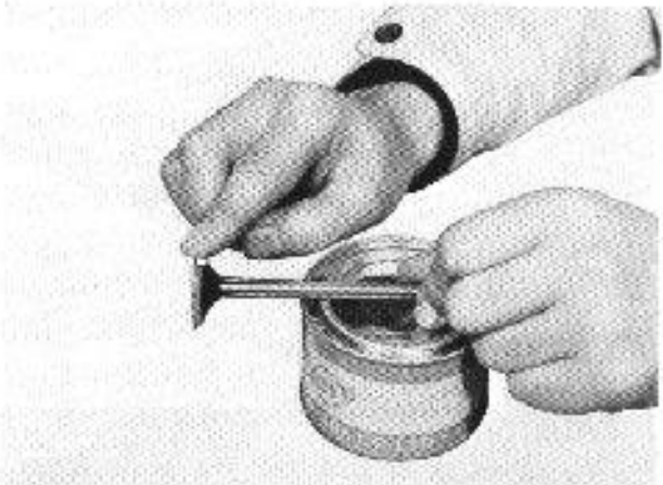
Fig. 3-69 Applying lapping compound to valve face
