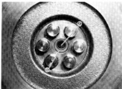
Fig. 11-9 ③ Oil seal, ④ Bearing
