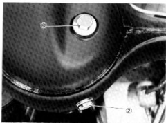
Fig. 16-32 ② Drain plug ③ Oil level plug
