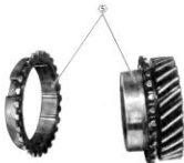
Fig. 13-21 ⑤ Checking contacting surface
