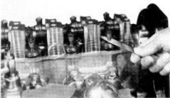
Fig. 3-151 Measuring valve clearance
