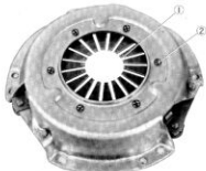
Fig. 11-7 ① Spring wear; ② Rivet
