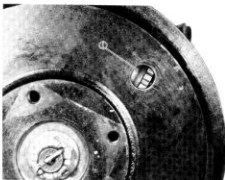
Fig. 14-24 ① Brake adjusting hole
