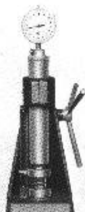
Fig. 3-72 Checking the spring for preload
