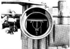
Fig. 4-6 Choke valve (with knob pushed in fully)
