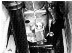
Fig. 13-38 ② Oil drain plug
